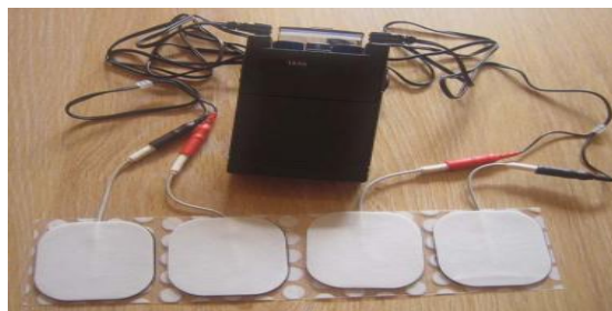
Gambar 2.1 TENS ( Transcutaneous Electrical Nerve Stimulator ). Sumber : Image courtesy of Wikimedia Commons.
