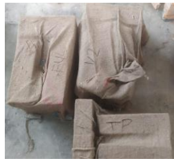
Gambar 3. 34 Perawatan Dinding Bata
