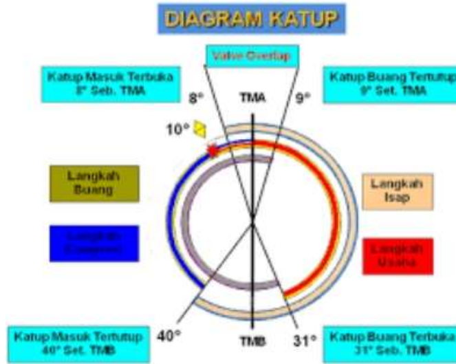
Gambar 2. 4 Diagram Valve
