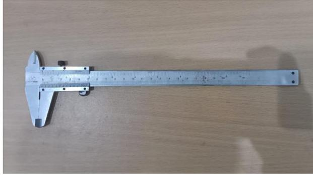
**Gambar 3. 13 Vernier Caliper**
