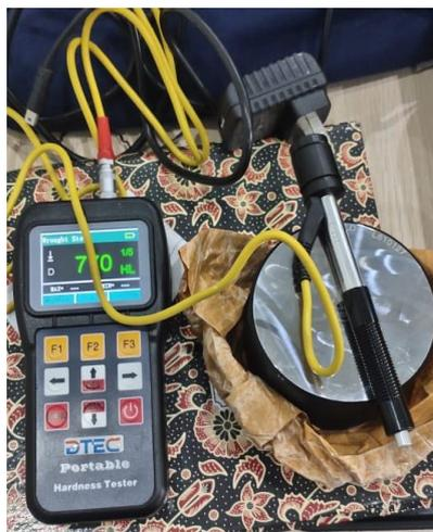
**Gambar 3. 25** Portable Hardness Tester
