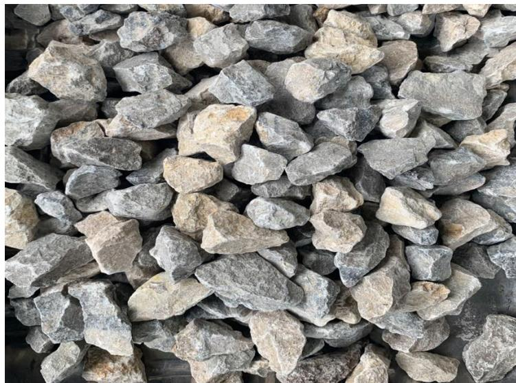
**Gambar 2. 2 Agregat Kasar Batu Gamping Loa Lepu**
