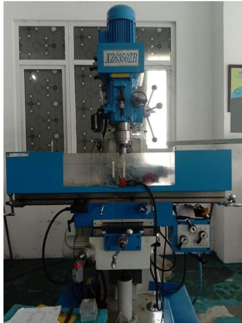
Gambar 3.3 Mesin *Milling* Konvensional
