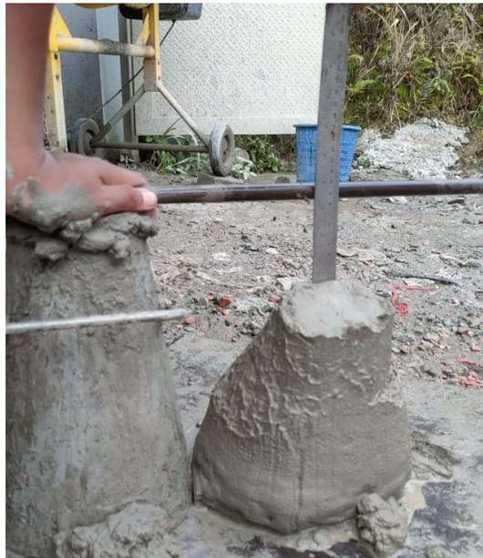
**Gambar 4.1** Slump Test Beton Prisma 10 x 10 x 30 cm
