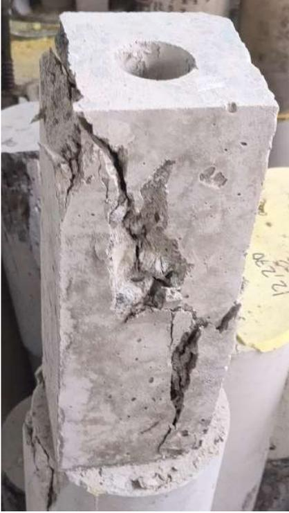
A photograph of a concrete prism specimen with a circular hole at the top. The specimen shows significant shear failure, with a large, jagged crack running vertically down the side, exposing the internal structure. The concrete is light gray and appears to be in a laboratory setting.                                              | <p>Beton Prisma Tanpa Pipa<br/>Variasi Lubang 1 ¼ inch<br/>Tipe Retak Geser</p>                |
