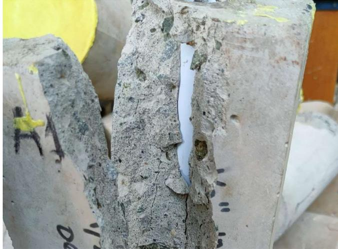
**Gambar 4.12** Hasil Zoom in Benda Uji Beton Prisma A1
