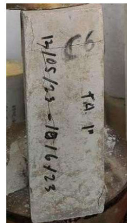
Figure 11. Prism Concrete Without Pipe 1 inch Hole Variation Shear Crack Type
