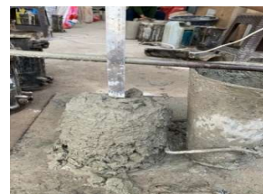
Figure 7. Slump Test for Concrete Source: Research (2023)
