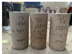
Figure 15. Concrete test specimen before being tested Source: Research (2023)
