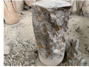
Figure 16. Concrete specimens, after being tested Source: Research (2023)
