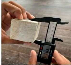
Figure 9. Measurement of the dimensions of a 5cm stone test object Source: Research (2023)
