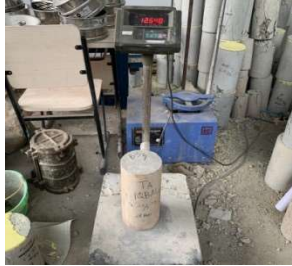
Figure 8. Concrete Test Specimen Weighing Source: Research (2023)
