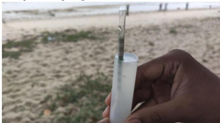
**Gambar 3.1** Pengujian kadar garam
