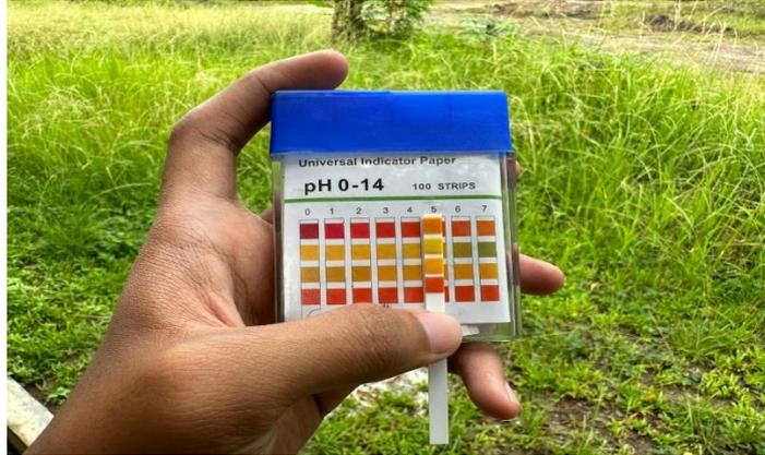
**Gambar 3.2** Pengujian kadar pH
