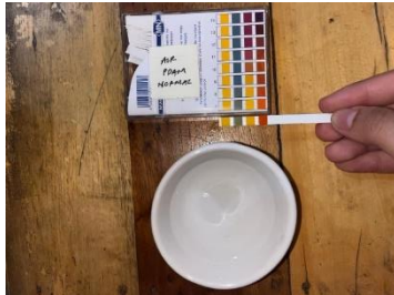
Gambar 3 Pengujian Air Normal pH 7,0
