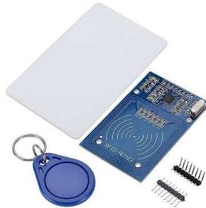
Gambar 1.1 Alat RFID Reader
