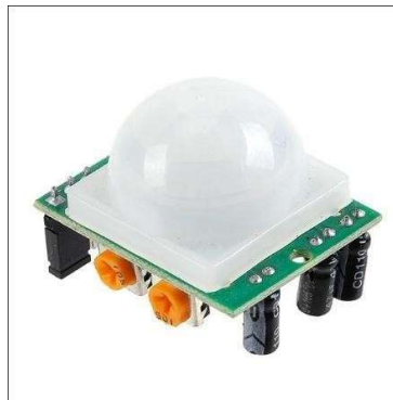
Gambar 2. 2 Sensor PIR (Passive Infrared Sensor)
